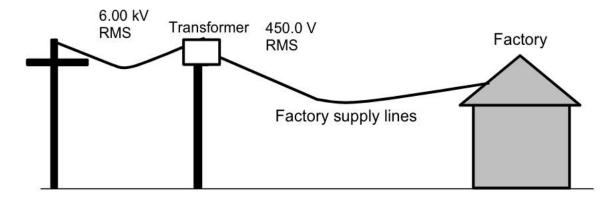
(a) Calculate the power loss in the factory supply lines.
